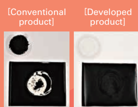
Chemical resistance test: Chemicals are applied, heated for 24 hours, then wiped off.
